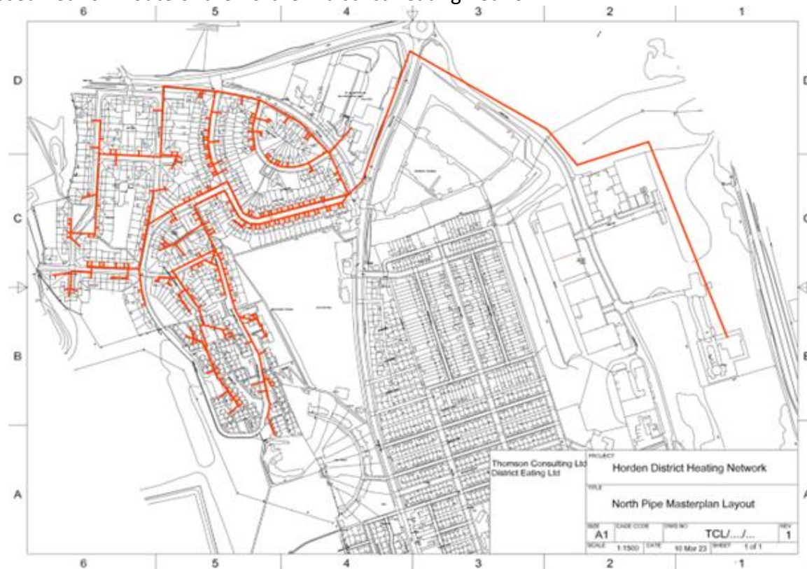
Figure 17: Northern district heating network
