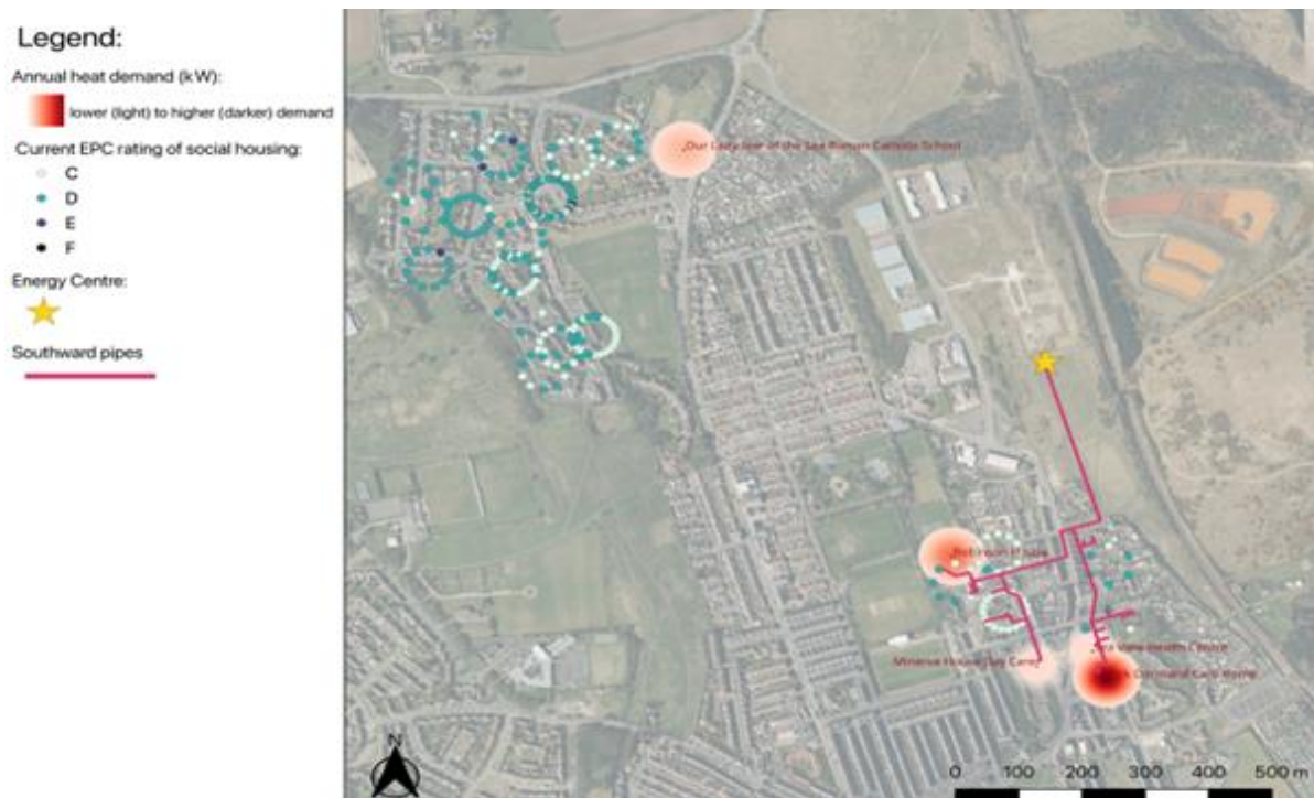
Figure 8: Heat mapping and network layout of scenario 1
