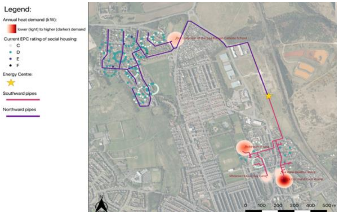
Figure 11: Heat mapping and network layout of scenario 2
